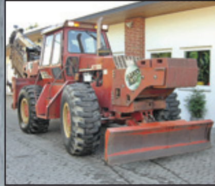
Ditch Witch RT 185, 4x4 , Bj. 2001, Kabine, Heizung, Panzerfräskette
